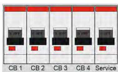
One pole circuit breakers for 120 V AC systems
